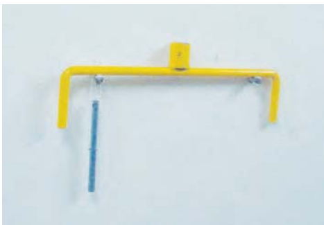
A removable hand-winding arm with brake release lever
